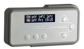
Active boost allows for a 1,2 or 3 hour heating boost at the selected temperature for when you just want a little extra heat, after the time period expires Dataterm reverts back to the plan loaded.
