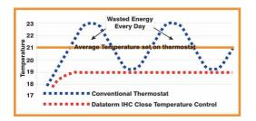
If you are comfortable at 19°C and an ordinary room thermostat is fitted it may not turn off until it peaks at 20 or 21°C due to inaccuracies and drop to 17 or 18°C before the boiler comes back on.
