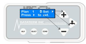
Use + key to temporarily raise the temperature & turn on heat.
